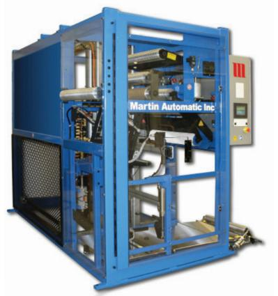
When the specified footage has been rewound, or upon a signal from the process or the operator, the web is transferred from the full roll to the empty core—without stopping or slowing the process. The full roll is lowered to a delivery ramp, the deflated spindle retracts, and the roll is unloaded—all automatically. The empty spindle returns to its core loading position.
